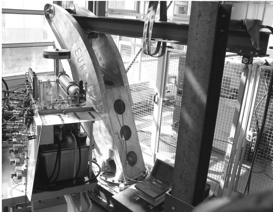
Fig. 10. Fatigue test on telescope arm support.
