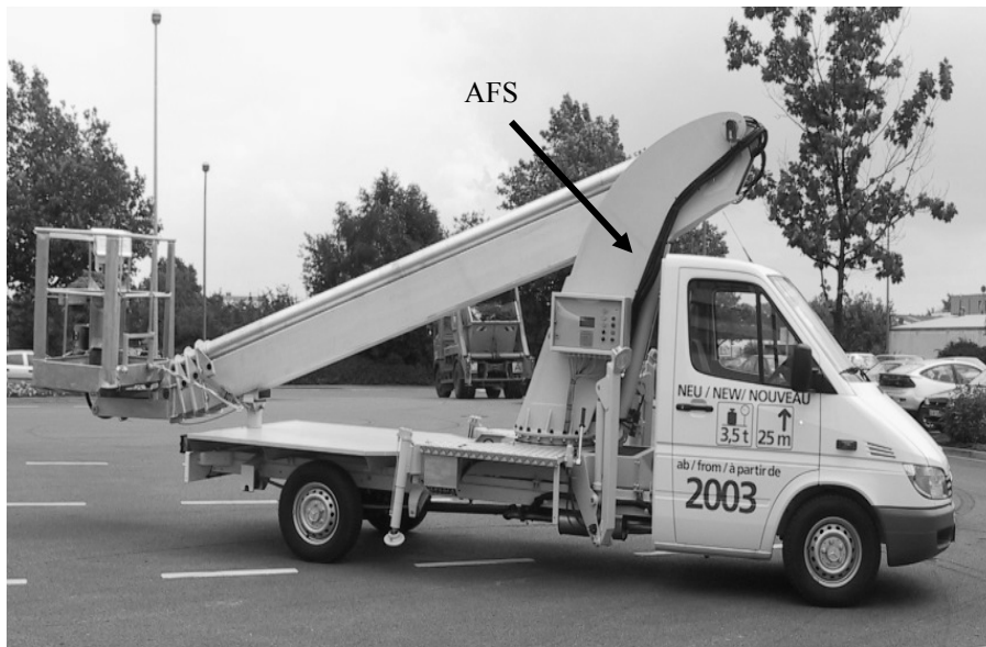
Fig. 6. Support of a working platform made of AFS.
